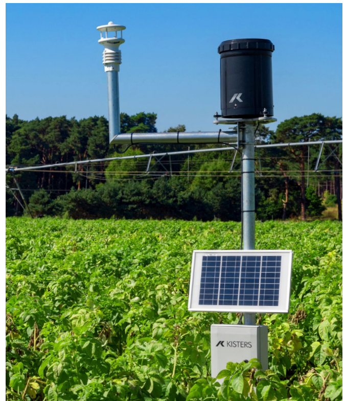
Figure: FieldRay station measuring environmental parameters for crop water balance analysis
